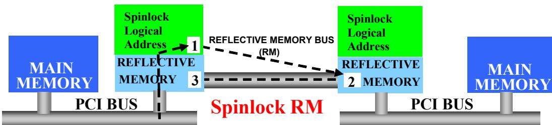
**Write to Spinlock address. Update the Remote Reflective address. Update the Local Reflective address when all remote node updates are completed.**
